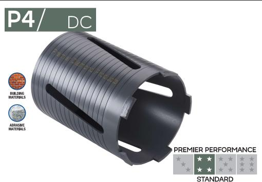
**DESCRIPTION:** Premier Diamond Products standard dry cores are suitable for drilling all popular building materials. The spiral barrel helps remove debris and increases air flow to the cutting edge while the diamonds and metal bond system, which were developed by Premier Diamond in 2004 especially for UK materials, provide fast, trouble free drilling. The P4 range may be our standard level, but their performance eclipses many premium products.
