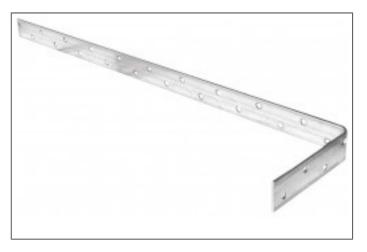
H and L straps are designed to The Building Regulations, BS 5268 Part 3 and other building standards for vertical and horizontal restraint when connecting timber floor and roof systems to masonry walls.
