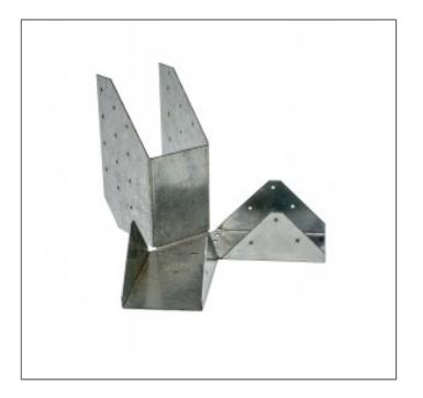
The HRC is a one-piece connector for supporting hip members from the ridge beam or rafters. It is site adjustable for slopes up to 45°, to cater for the hip pitch for both left and right rafters.
