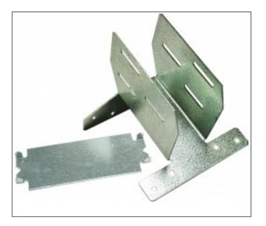
Glide shoes are specially designed to allow horizontal movement between raised tie trusses and wallplates. The GS allows lateral movement of raised tie trusses up to 15mm during installation of roofing materials and resists uplift forces. Typically used on one or both ends of the truss as determined by the truss designer.
