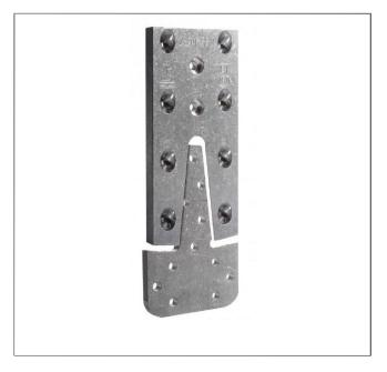
The first part of the connector is fixed into a pocket on the header timber with nails and the second part is fitted on the end of the in-coming beam with screws.
