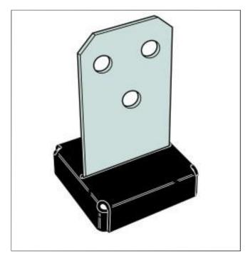
The CPT concealed post base provides a clean, concealed look while providing a 25mm standoff height above concrete. The 25mm standoff reduces the potential for decay at the post end. The CPT can be fixed to concrete base with either M12 chemical or mechanical anchors (sold separately).
